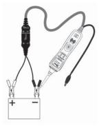
While the PP3 is in Power Probe Mode. Contact the probe tip to a <a href="MEGATIVE">MEGATIVE</a> circuit. The green negative sign "- " LED will light. If the audio feature is turned on, a low pitched tone will sound.
