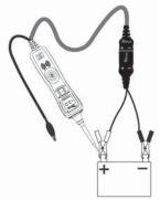
While the PP3 is in Power Probe Mode, contact the probe tip to a POSITIVE circuit. The red positive sign "+" LED will light and the voltage reading of the circuit will be indicated on the LCD display. If the audio feature is turned on, a high pitched tone will sound.
